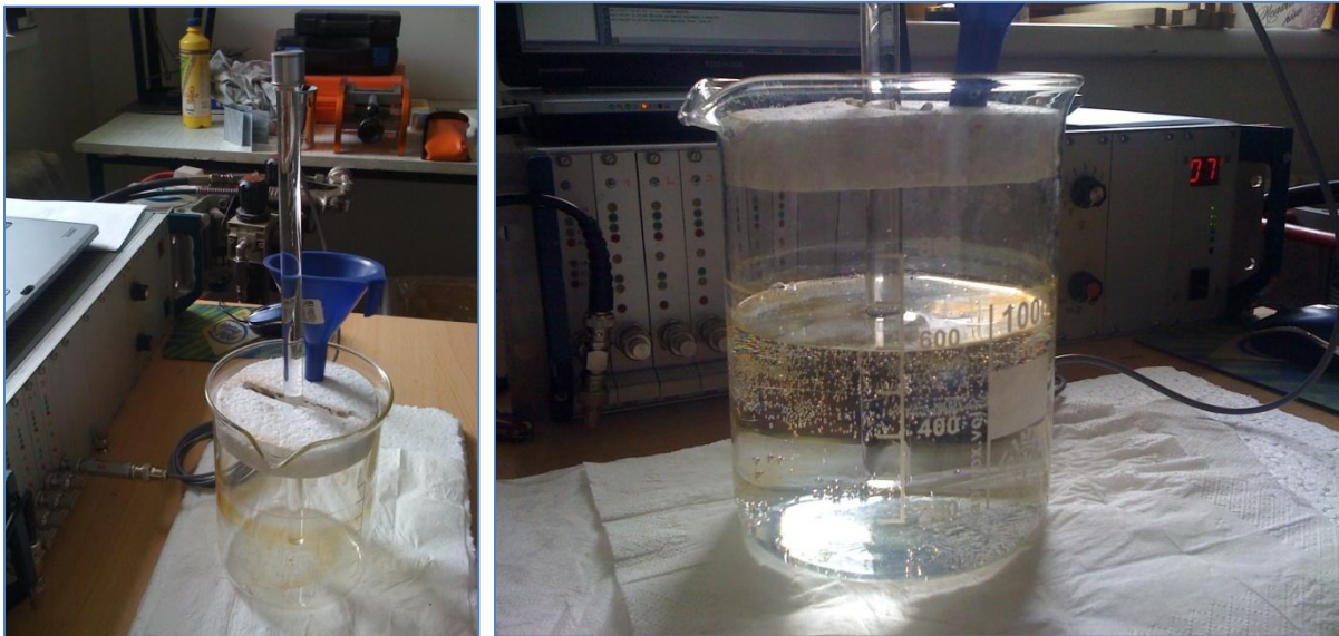
Figure 4. Testing glass-rod waveguide immersed in the water. Note the blue filler inserted in the polystyrene lid. Photo by David Varner.
