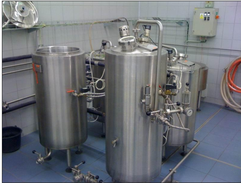
Figure 1. Cylindroconical fermenter in the Destila micro-brewery. Note the observation opening on top surface. Photo by David Varner.
