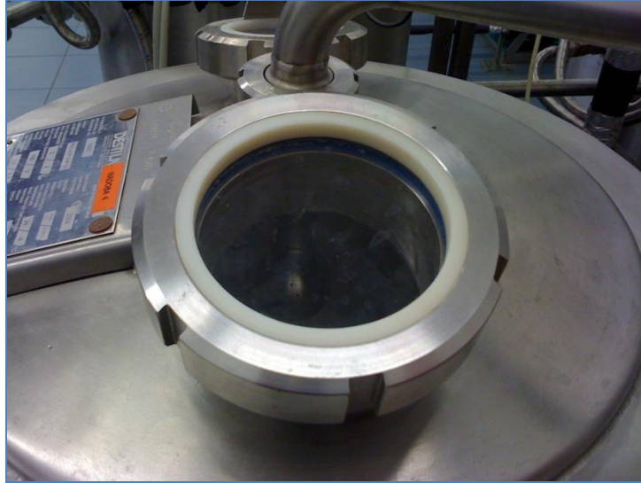
Figure 2. Opening on the tank body with original glass lid. A new glass-rod waveguide assembly will be inserted instead of the glass. Photo by David Varner.
