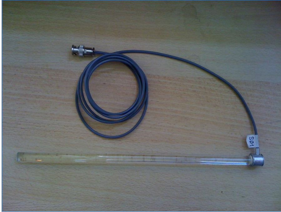
Figure 3. Test glass-rod waveguide with piezoelectric AE sensor attached. Photo by David Varner.
