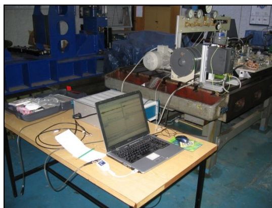
Figure 3 Control PC with Dakel Daemon software and hydraulic circuit with the pump.
