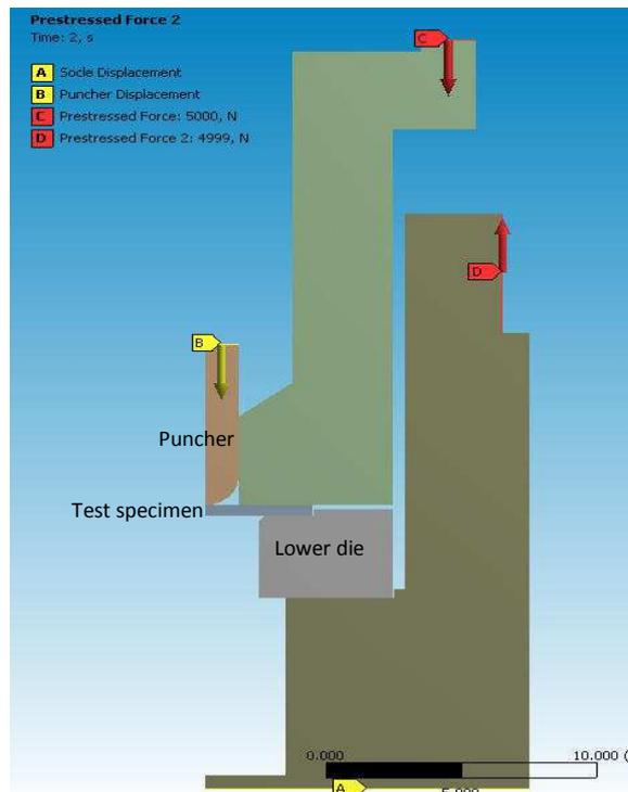
**Fig. 1:** Geometric model of PD
