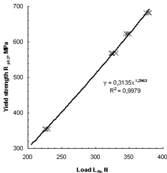
Fig. 6: Procedure of "yield load"  $L_{Re}$  assessment
