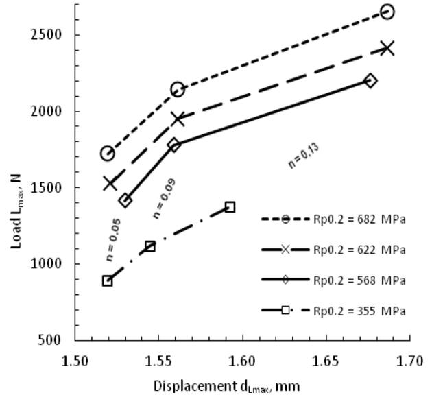
Fig. 3: Effect of yield point and hardening on SPT results
