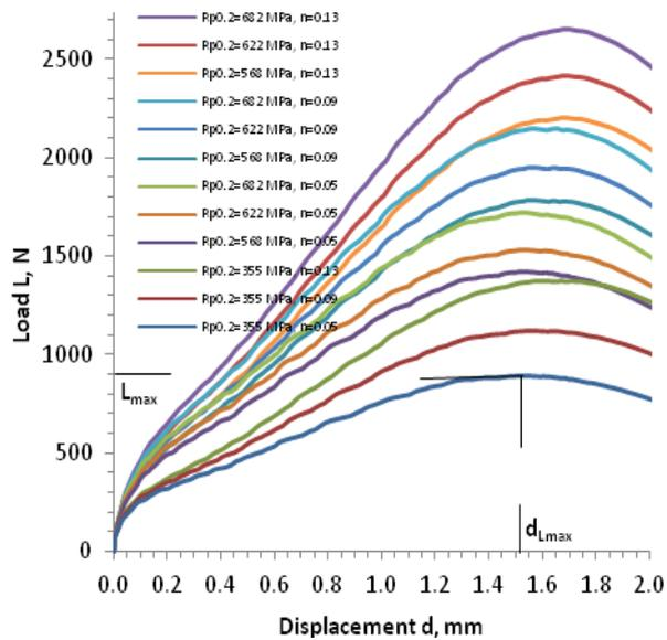
Fig. 2: Load-displacement curve for model steels
