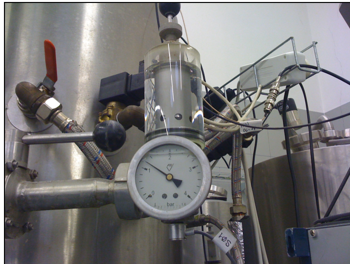
Figure 3: Position of SENSOR2 on the bottom of the carbon dioxide outlet valve assembly. Photo by D. Varner
