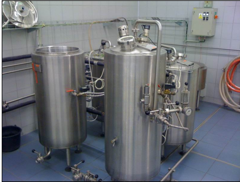
Figure 1: Fermentation part of Destila micro-brewery facility. The cylindroconical fermenter is in the foreground. Photo by D. Varner
