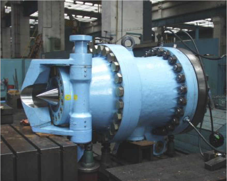
Fig. 12. Straight flow nozzle during pressure test
