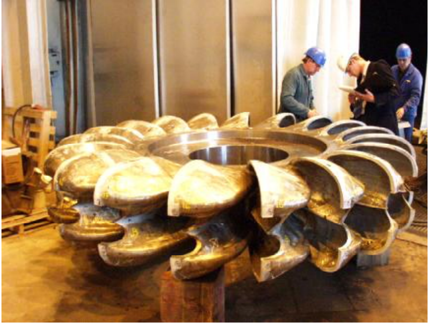
Fig. 11. Tillari - casted runner during inspection
