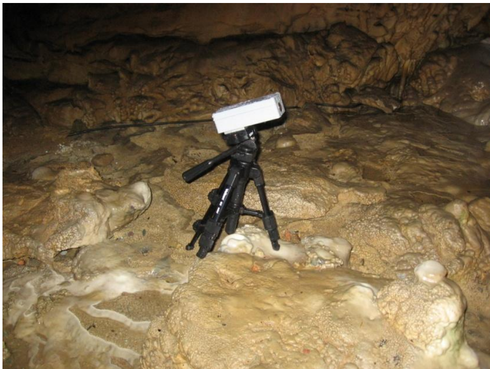
Figure 04: Dropmeter in "combat" position in the cave. Note the adjustable tripod and non-horizontal setting of the device. Photo by David VARNER
