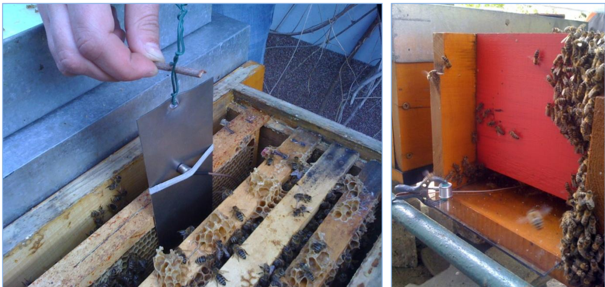
Figure 05: Slot01 sensor on the sheet metal plate. Photo by David VARNER
