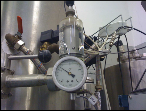
Figure 3: Position of SENSOR2 on the carbon dioxide outlet valve assembly. The sensor can be seen below the gauge dial, glued upside-down to the bottom of the assembly. Photo by D. Varner
