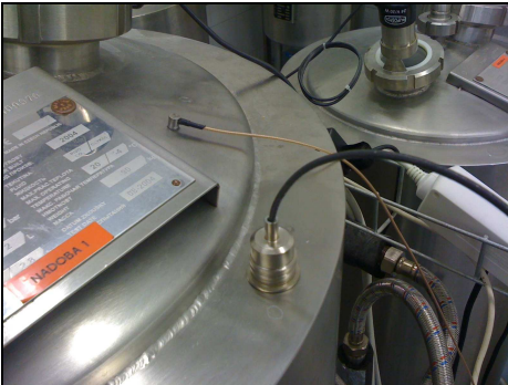
Figure 4: Position of SENSOR3 on the top of the fermentation tank (the small one, in background). In the foreground, a big calibration sensor is temporarily glued to the double-wall portion of the tank. After successful calibration of the AE monitoring assembly, it was removed. Photo by D. Varner
