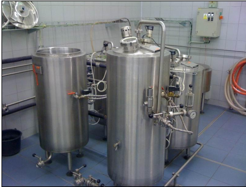
Figure 1: Fermentation part of Destila micro-brewery facility. The cylindroconical fermenter is in the foreground. Photo by D. Varner
